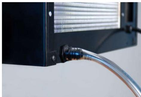
Our **REAR** drain line comes with the fitting installed in the rear of the cooling unit. Our **BOTTOM** drain line requires installation of the fitting. To install, apply pipe joint sealant (included) to the male threads of the barbed fitting, then hand-tighten the fitting into the threaded drain line hole. Do not force – if cross threaded, back out and realign. Finish by tightening the fitting with a wrench.
