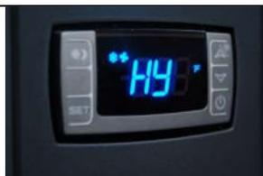
**TEMPERATURE DIFFERENTIAL:** The factory preset for this setting is “4”.
