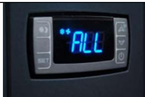
**LOW TEMPERATURE ALARM:** The factory preset for this setting is “45”.
