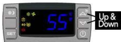
To reset the “High Temp” or “Low Temp”, press the “Set” button for three seconds while “Hi” or “Lo” is displayed. **“RST” will blink three times to indicate confirmation.**
