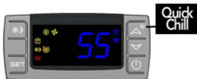
To activate the "Quick Chill" mode, press the "Up" / "Quick Chill" button for three seconds. To deactivate "Quick Chill", press "Quick Chill" button for three seconds again
