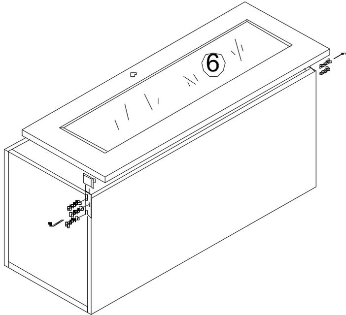
With cabinet on back, place the door on frame. With just the weight of door gaskets tighten hinge bolts in place.
