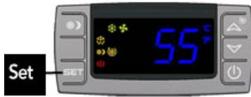
Minimum Set Point of 58°F and a Temperature Differential of 4°F. This means that the cooling unit will turn on when the display rises above 62°F (58°F + 4°F), and turn off when the display falls below 58°F.
