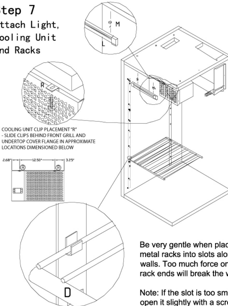
Be very gentle when placing metal racks into slots along walls. Too much force on the rack ends will break the weld.
