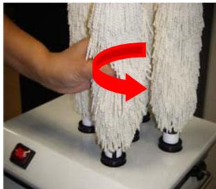
To remove the brush from the support, rotate the brush in a counter clockwise direction while gently pulling it upwards. Remove the brush completely by slipping it off its support.
